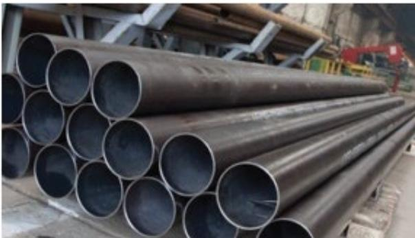
Steel pipe has long been used in a versatile range of construction applications. It balances structural strength and density with ease of fabrication, is non-combustible, offers a wide range of coating options, provides close tolerances for wall thickness, resists damage from heat and pressure, and delivers long product life. Steel is another highly reused and recycled material in the construction sector with a recycling rate of up to 94% according to the Steel Recycling Institute.
