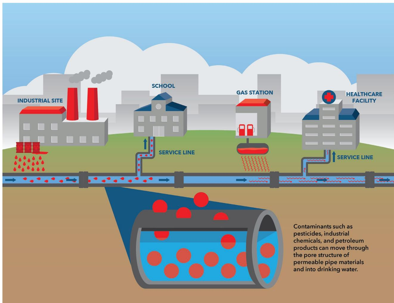
Piping that connects buildings to water mains often passes belowground, under streets or through soil that may have contain environmental pollutants such as petroleum products, pesticides, industrial waste, or other chemicals. Research shows that many commonly used pipes can allow these substances to pass through the piping walls, a process called “permeation.”
