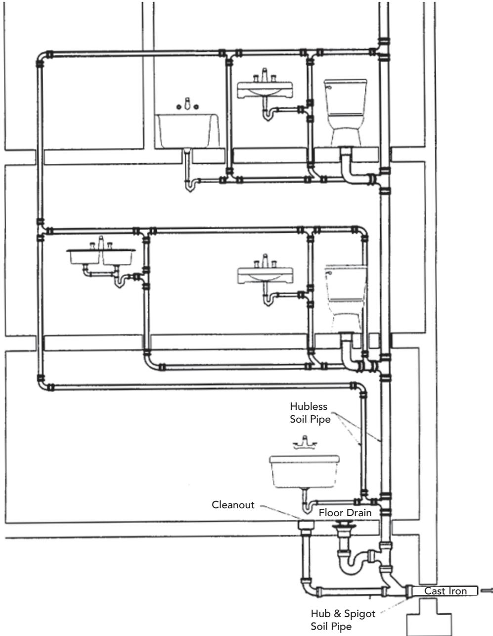
Vent pipes complement drain/waste systems by allowing mixtures of liquid and solid waste to flow easily down pipes while preventing siphonage and backflows. Vents also carry away gases and fumes associated with waste, venting it to the exterior and safeguarding interior air quality. Branch vents connect most if not all individual drains and piping segments of waste systems to main vent stacks.
