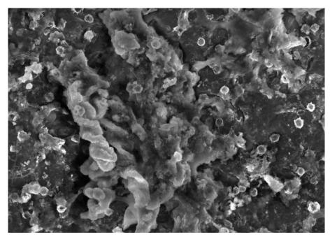
"Environmental, chemical & biological factors can degrade PE pipes"
